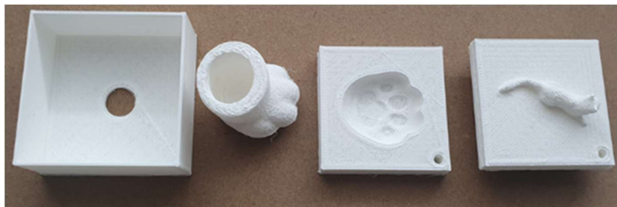
Figure 9. 3D model of an aid for identifying a domestic cat using its footprint, printed on a 3D printer
