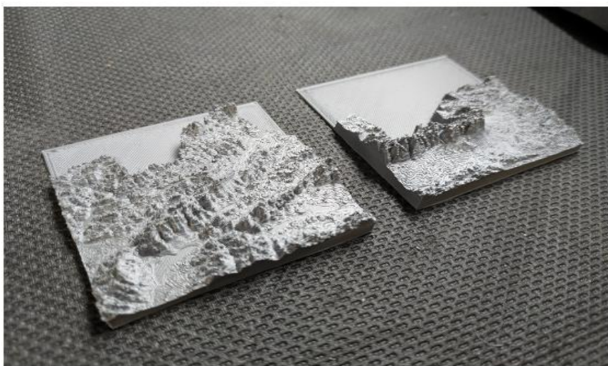
Fig. 76 Detail of the relief of the 3D map of Slovakia after printing
